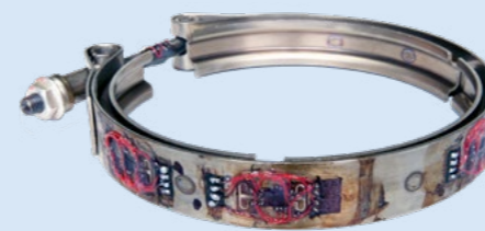
Strain Gauge Application on Clamp
