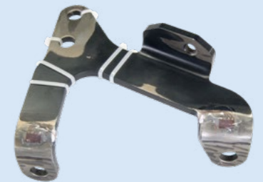
Strain Gauge Application on Holding Bracket
